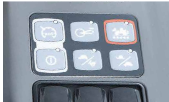
Controller: Variable key fields for driving and working
